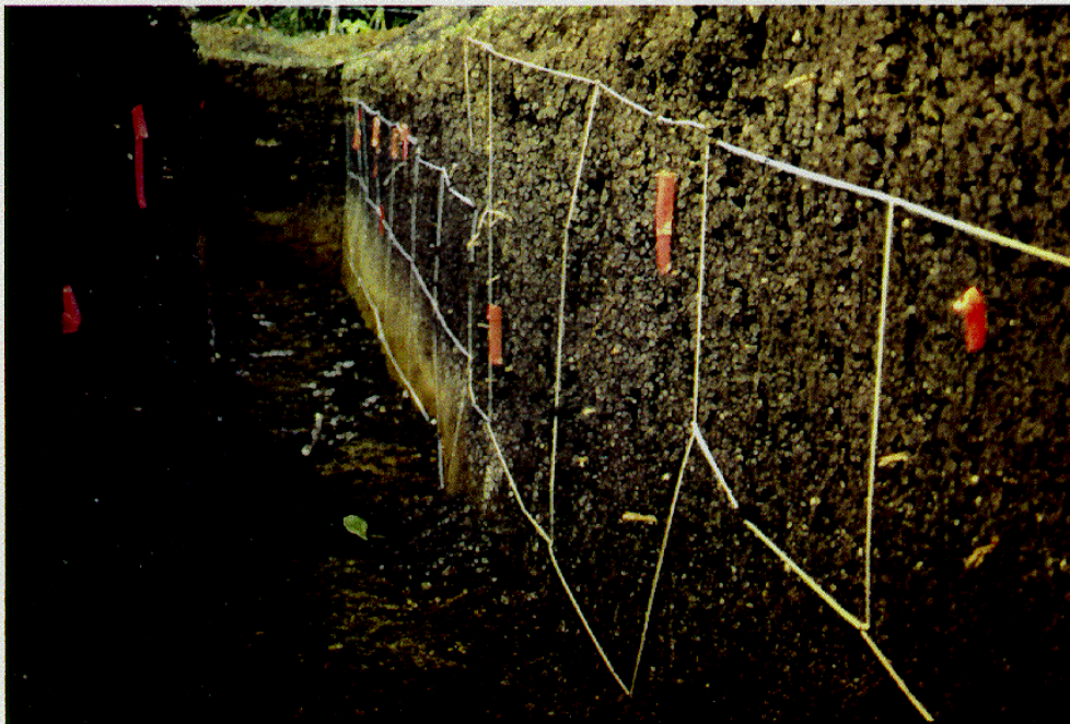
Figure G-4: Photograph of Trench RJJ showing T1 fluvial deposits (bottom of trench in distance) and overlying pond deposits (unit 40).
